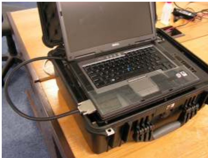
Figure 4, Switch on RS machine and connect it with laptop before turn on laptop
