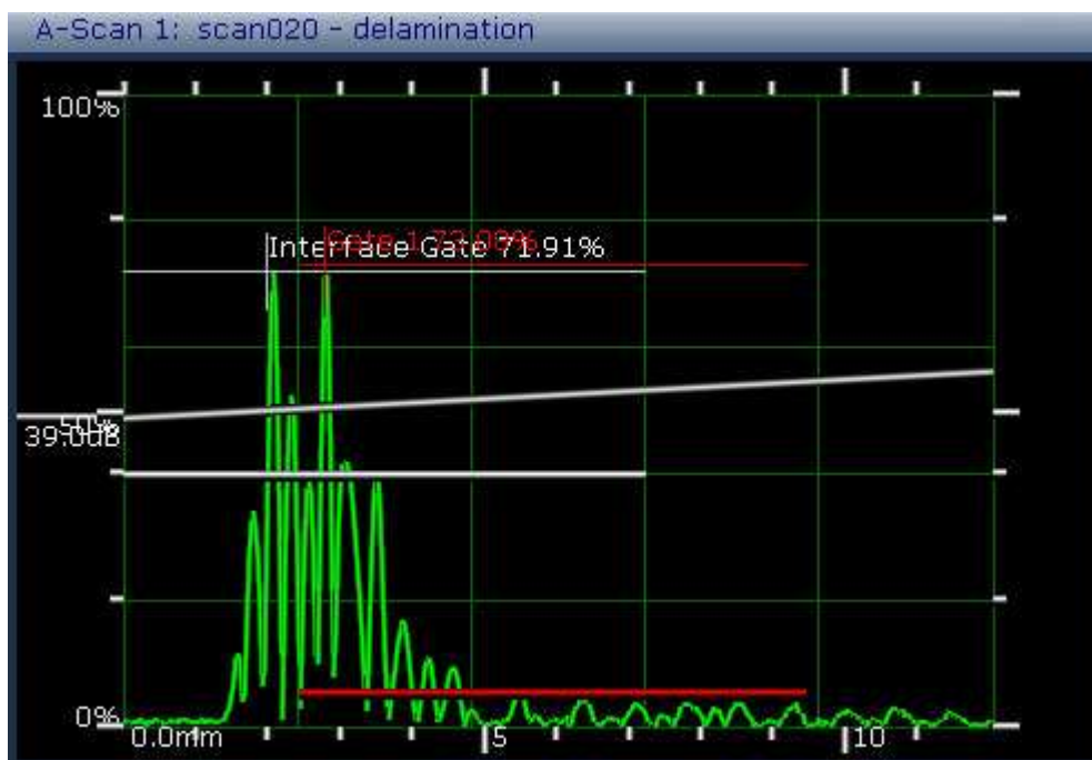
Figure 84: A-scan from a near surface defect (0.7mm depth)
