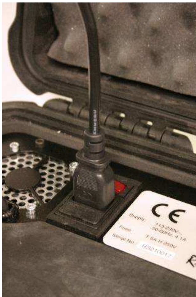
Figure 13: RapidScan Power Cable Connector
