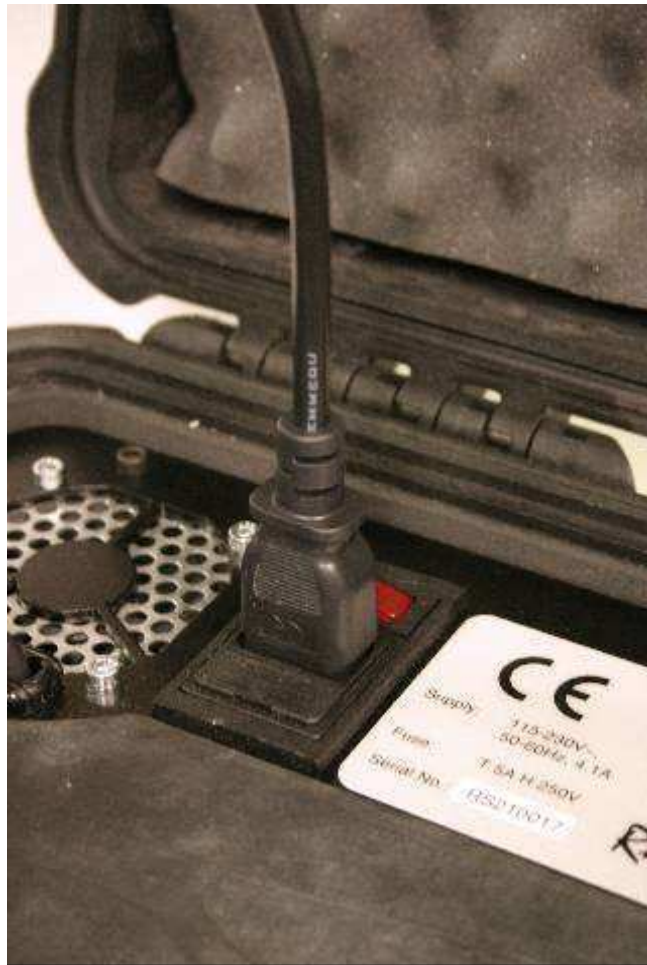
Figure 6: RapidScan Instrument Power Connector
