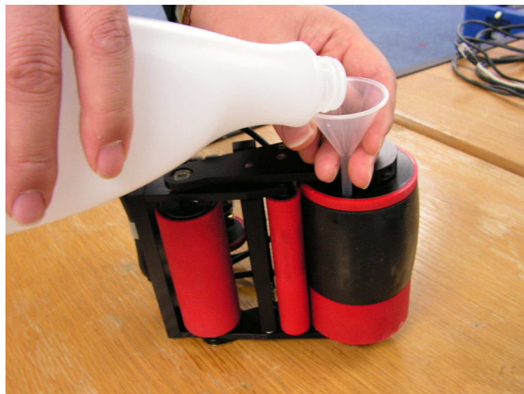
Figure 8: Filling Wheel Probe Tyre with Water
