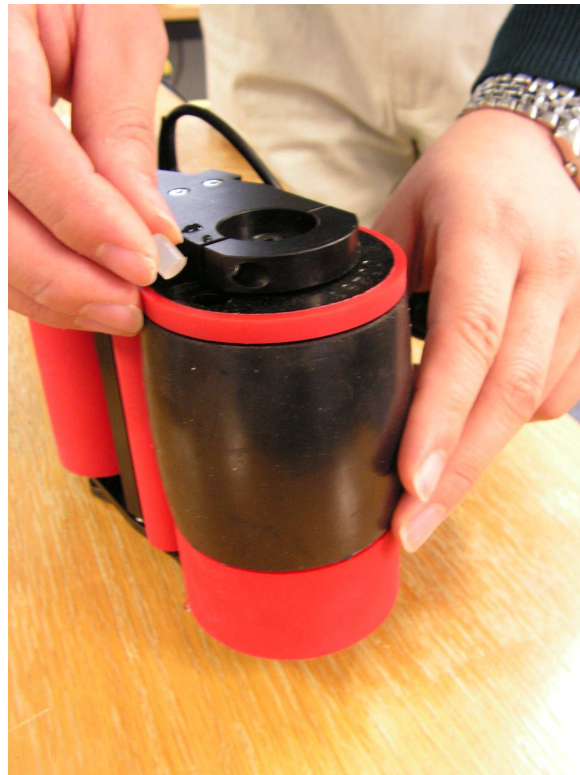
Figure 7: Removing Wheel Probe Bungs
