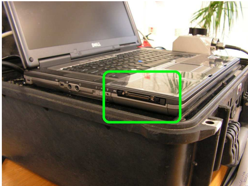
Figure 2: An attached but unconnected adapter card.
