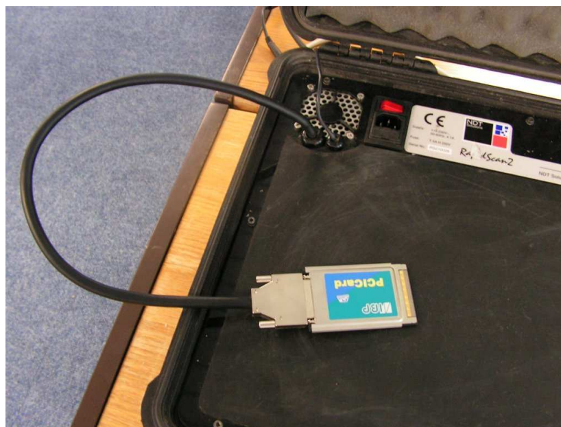
Figure 3: A correctly connected adapter card and RS instrument
