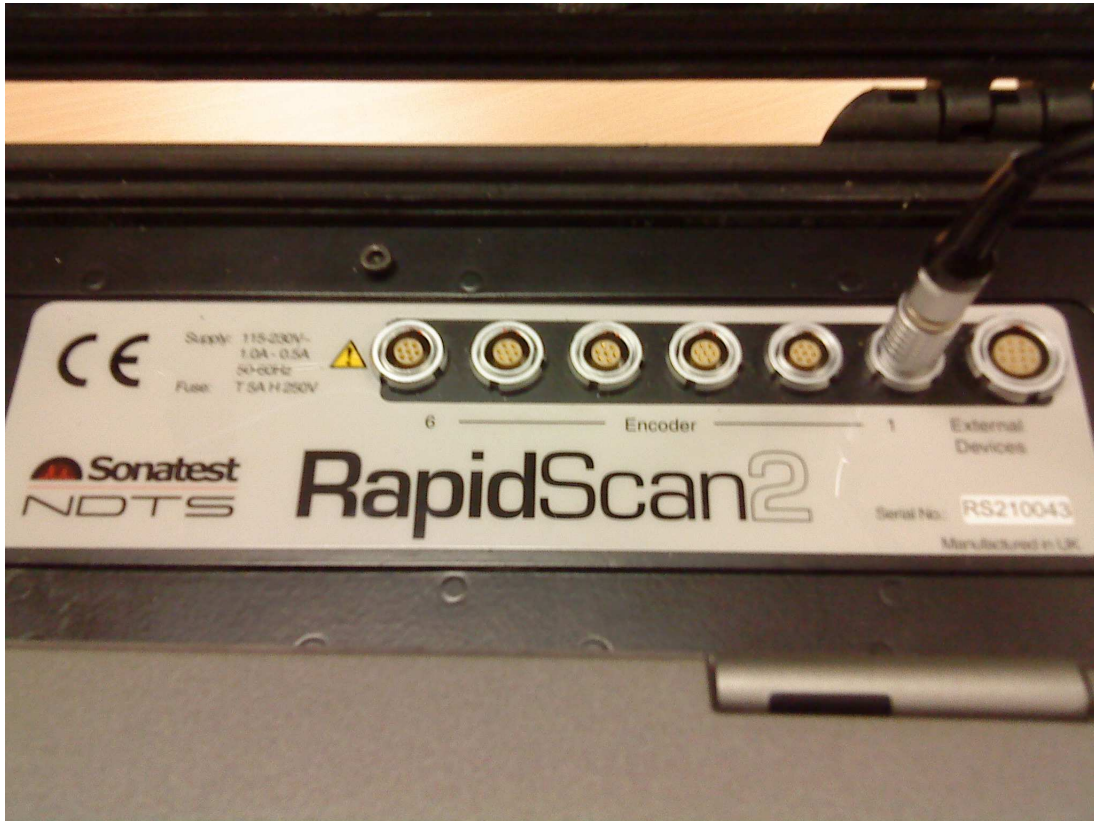
Figure 10: RapidScan2 Position Encoder Connector
