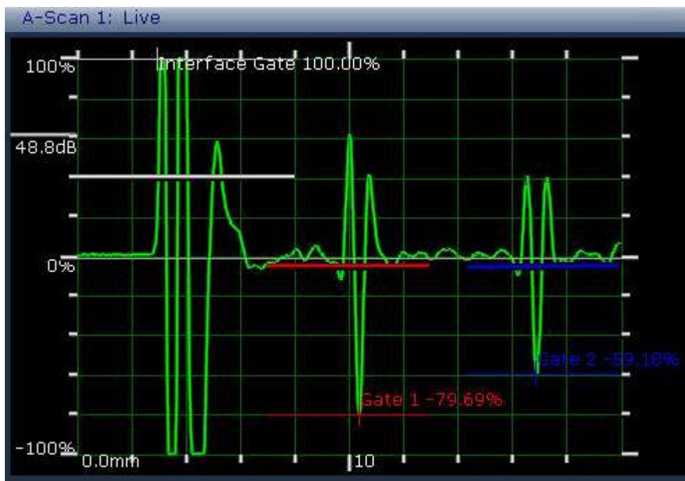
Figure 111: A-scan showing gate set up
