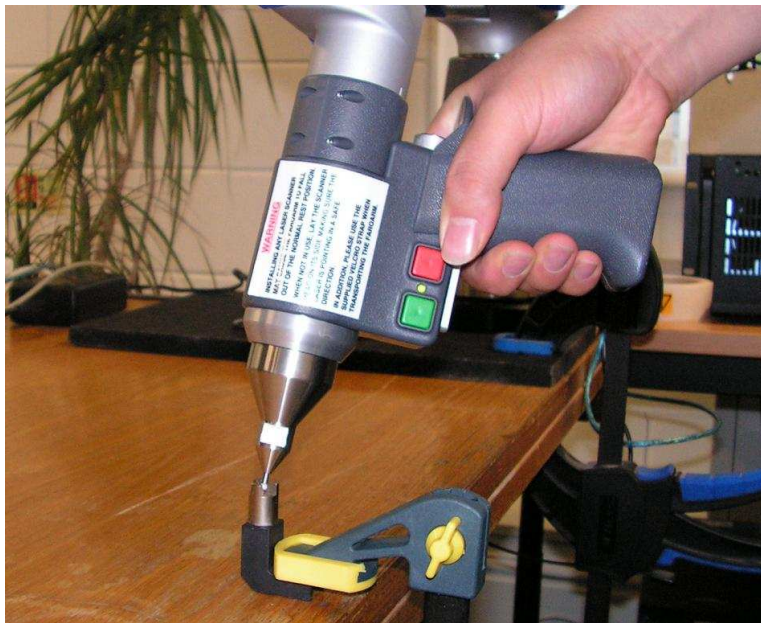
Figure 28: Almost completed collecting first set of points for hole calibration
