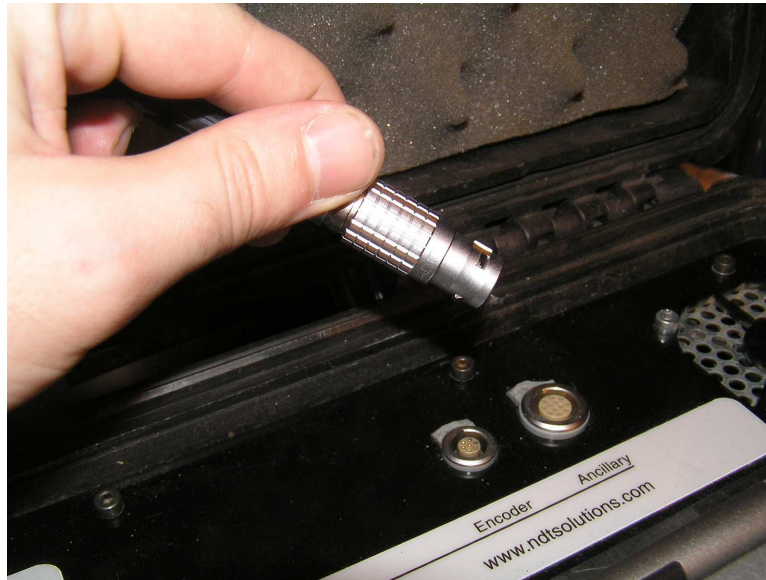
Figure 11: RS3D sync cable connection for instrument
